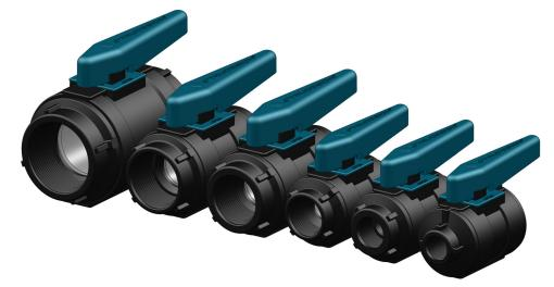
The body of the Ball Valve is manufactured in a glass reinforced nylon composite with high impact and tensile strength resulting in a light weight unit, free from corrosion and electrolysis issues. The ball and sealing rings utilise a PTFE polymer to ensure a smooth action, and continuous ease of operation over many years.
